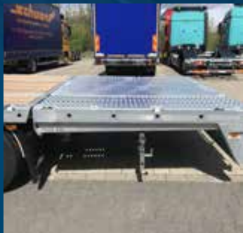
Hydraulically lowerable rear with 5.5 t lifting force
