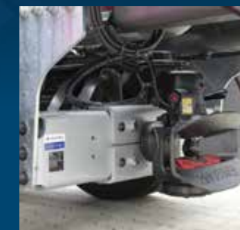
Pneumatic deep coupling system with remote display
