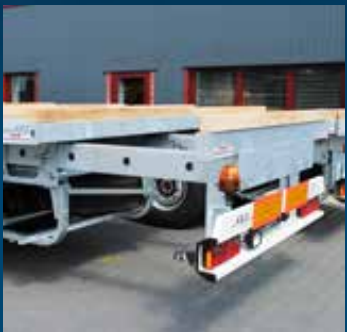
Rear extension with roller bearings
