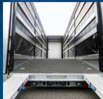
Semi-trailer with lowerable rear and drive-on ramps
